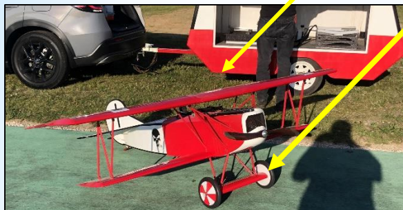
Dan Vensel's custom trailer and Fokker biplane with 22" prop, two 6 cell lipos in series, and 24 lbs.
